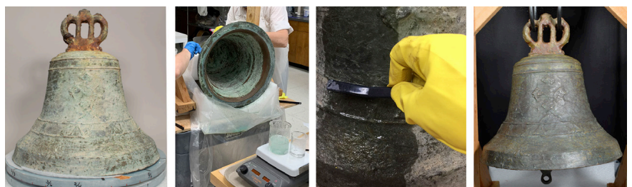
Figure 4. San Agustín bell: (a) before treatment, (b) during cleaning, (c) brush detail, (d) after treatment
