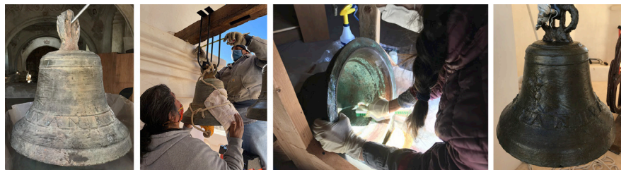
Figure 1. San Pedro bell: (a) before treatment, (b) during cold waxing, (c) after treatment
